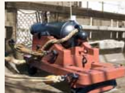
Left: Naval cannons on truck carriages; right: a carronade on a pivoting slide carriage.
